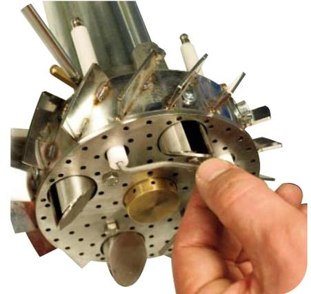
**10-** Reassemble the ignition electrode screwing the screw with the spanner.
