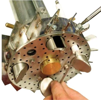
**9-** Reassemble the ionisation electrode screwing the screw with the spanner.
