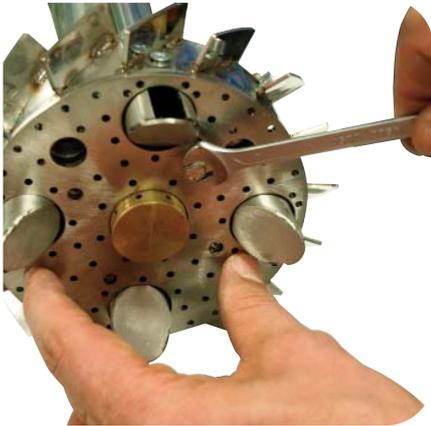
**8-** Install the disc with nozzle screw the 4 fixing screws with a spanner.
