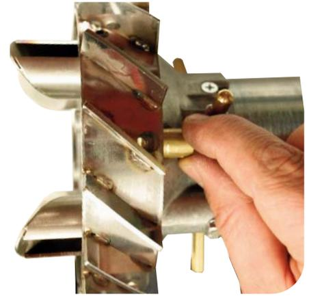
**7-** Introduce the bushings of electrodes.
