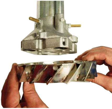
**6-** Install the rear disc and reassemble the diffusers screw the fixing screw with a screwdriver.
